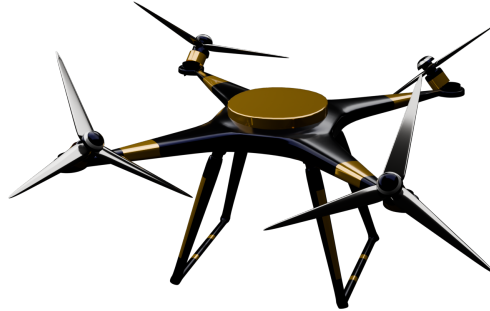
Figure 7.2. CAD rendering of the tilted quadrotor prototype.
